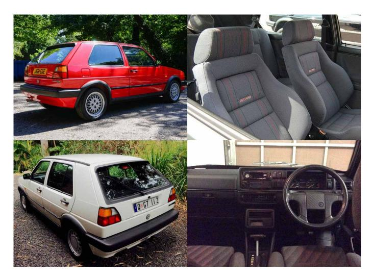
All early MK2's had a fuel injected 1.8L 8v engine putting out 110bhp driving the front wheels through a 5 speed gearbox. These early MK2s can be identified from later cars as they feature small bumpers, quarter windows in the front doors and LHD wipers. They can be identified form MK1 Golfs by the rear lights (triangular rather than square), a swage line behind the rear window and generally bigger in size.
